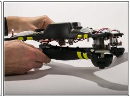
Cut the yellow strips using a scalpel. Pry open the casing using pry tools working gently around the corners.
