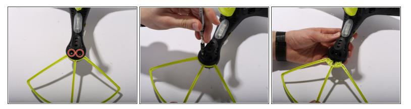
Remove Blade Guards by unscrewing two 13 millimeter screws using Philips #0. Pull out the guards. Repeat the steps for the other three corners.
