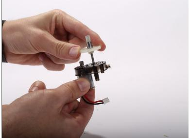
Slide the pinion gear off of the motor assembly.
