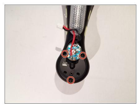
Remove 3 9mm screws around the motor housing. Repeat the steps for the three other arms.
