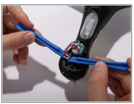
Unclip the motor cable from the shells housing using two pry tools. Repeat the same procedure for the other three arms.
