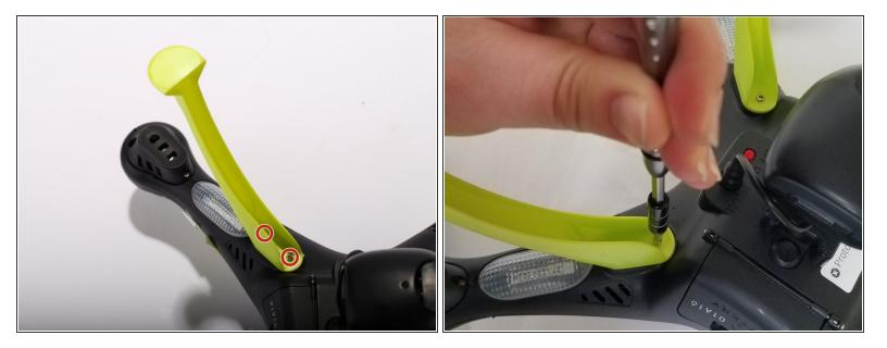
Unscrew two 9 mm screws located inside the legs. Repeat the same procedure for the other three legs
