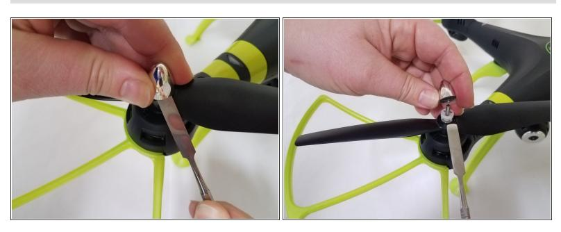
• Use the heavy duty spudger tool to pry off metal caps by pushing the spudger up into the cap.
