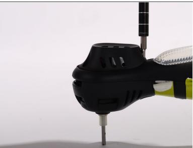
Remove the motor protection cover by unscrewing two 9 mm screws using Philips #0. When the screws are off, use your fingers to pull the motor protection cover off. Repeat the procedure for the other three arms.
