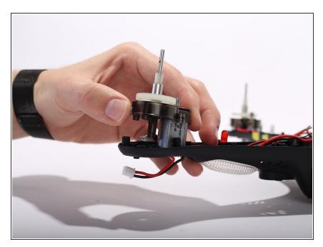
Remove the motor assembly from the bottom shell.
