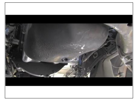
Allow the engine oil to drain for an extended period, such as 30 minutes, to ensure maximum oil removal.
