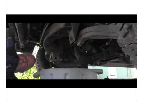
With the steel guard removed, locate the engine oil pan and use a 14mm socket wrench to remove the drain plug.
