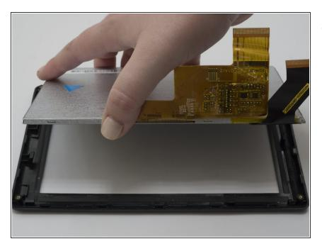
• Remove the screen from the frame by lifting it from the side.
