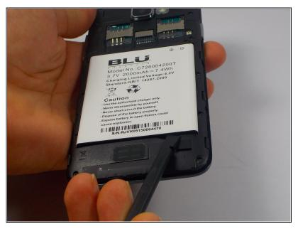
With the back panel off, you should see a large white rectangle. This is the battery. Slide the spudger under the indent on the bottom right of the battery and pull it up.
