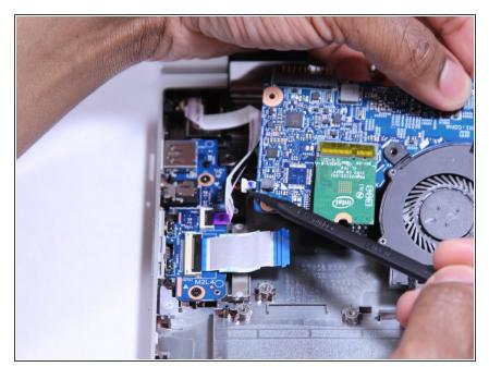
Using a Heavy Duty Spudger, disconnect the black and red RTC battery cable on the left side of the system board (motherboard).
