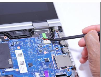
Disconnect the fastened cables from the system board (motherboard) by carefully pushing the cable's plastic edges using the Heavy Duty Spudger.
