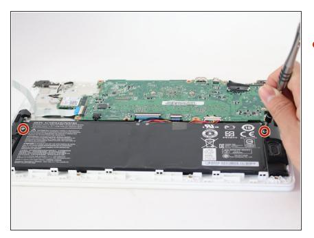
Locate and remove the two 6mm screws holding the battery in place with a Phillips #1 screwdriver.
