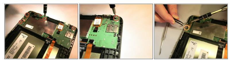
Using the Phillips #000 screwdriver, remove the four M1.4 × 2.5 screws holding the motherboard in place.
