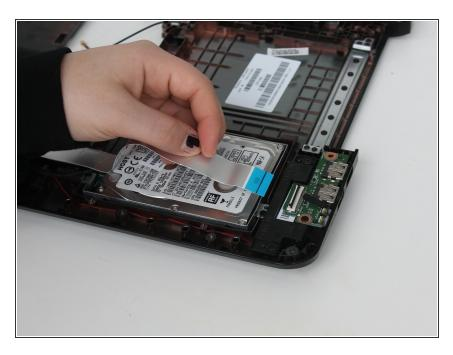
Disconnect the ribbon cable in the bottom right corner of the laptop.
