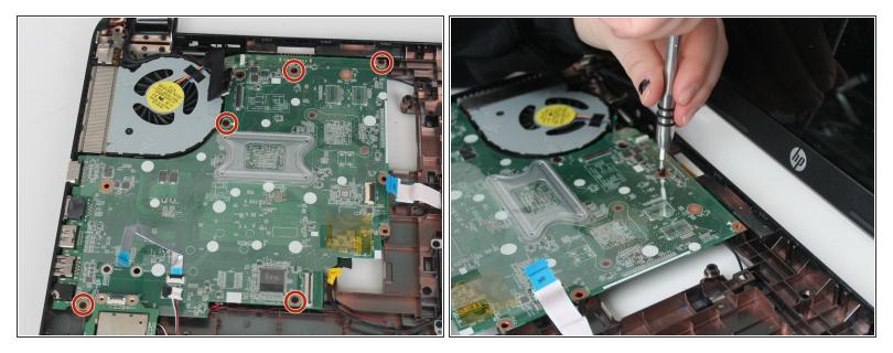
• Remove the five Phillips PM2.5×5.0 screws on the motherboard.
