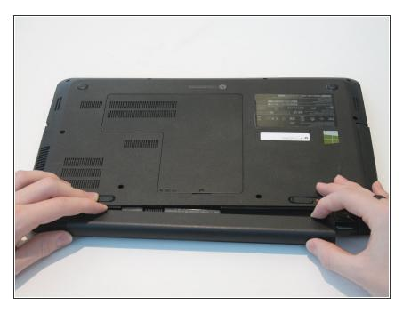
While holding the left switch in place, slide the battery towards you and away from the laptop.
