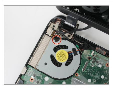
Remove the Phillips PM2.5×5.0 screw located on the fan, in the upper right corner.
