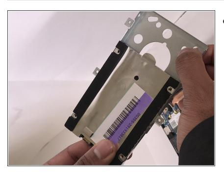
Pull the hard drive out of the metal frame.
