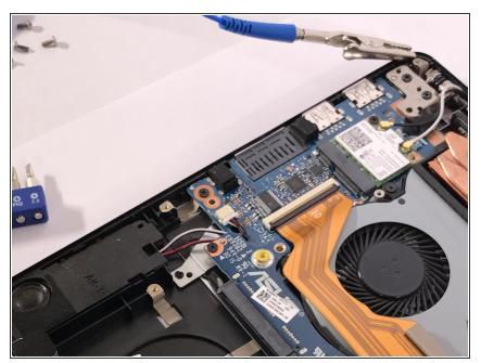
Attach anti static wrist guard to your hand and secure clip to the laptop case.
