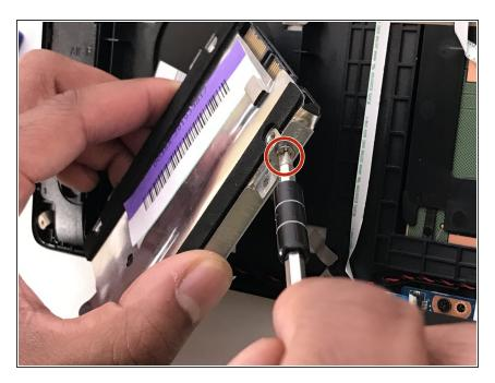
Using a Phillips 1 screwdriver, unscrew the four 4.5 mm screws from the sides of the hard drive.
