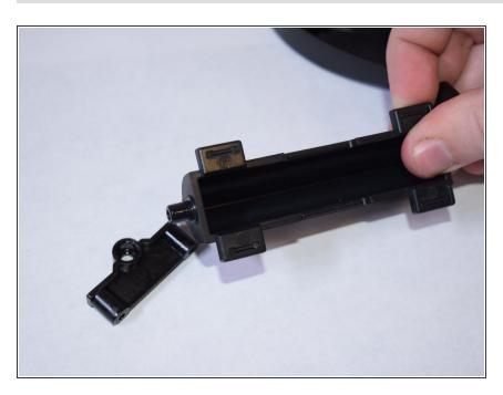
Once the Strum Bar is removed, there is a rectangular piece on the end which can be removed to apply lubricant if needed.
