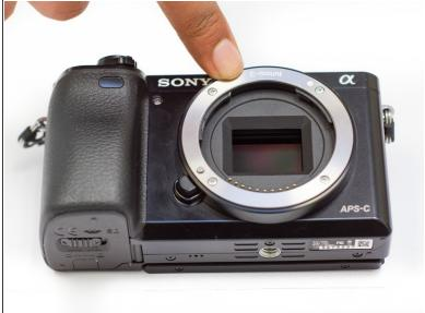
Locate the E-mount on the front of the camera
