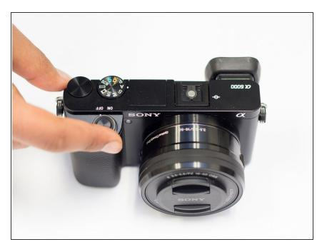
Turn of camera by turning the switch to OFF.
