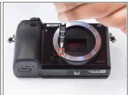
Take a Philips head 00 screw to remove the four of the 5.1mm screws located on the E-mount.
