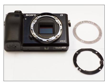
Replace the plastic E-mount ring with a new one.
