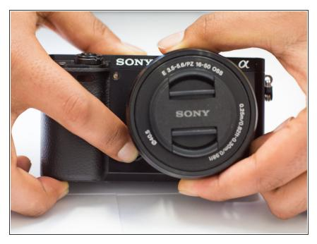
Use the finger, press and hold the release black circle button (on the bottom) next to the lens on the front of the camera.
