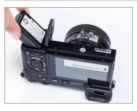
Once the battery is free, you are able to take the battery out of the compartment. The battery can now be replaced the battery with a new and fully charged one.
