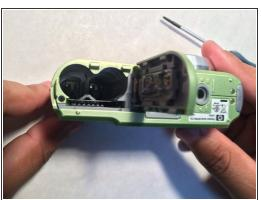
Disconnect from all power sources. (Remove batteries, chargers, etc.)
