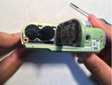
Remove the five 5mm screws from the bottom of the camera with a PH00 screwdriver.
