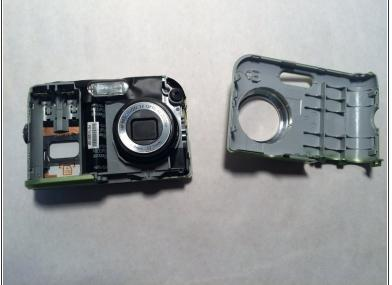
Make sure that the siding is fully removed and the battery dock is open. Carefully pry the top off of the camera.
