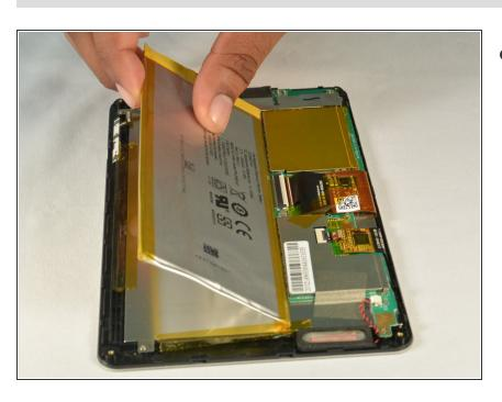
Lift the battery from the device.
