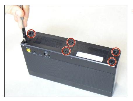
Locate the six 9 mm screws on the bottom of the SRS-X55 and remove them using a Phillips head #2 screwdriver.
