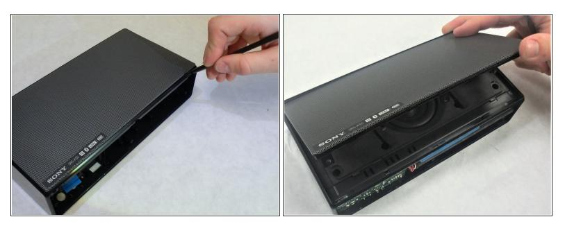
Insert a plastic spudger into the seam of the metal speaker cover and pry it downward until it releases from the speaker body.
