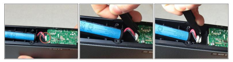
• Locate the battery plug and remove it using a pair of tweezers.
