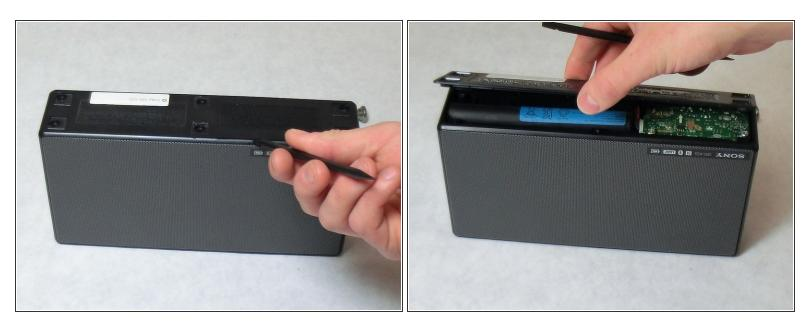
• Insert a plastic spudger at the seam of the bottom panel and remove it from the rest of the speaker.
