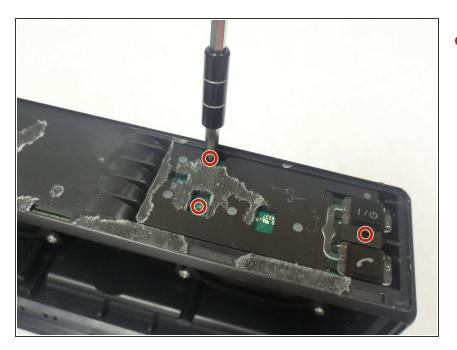
Locate the three 4.5 mm screws on top of the speaker input board and remove them using a Phillips head #2 screwdriver.
