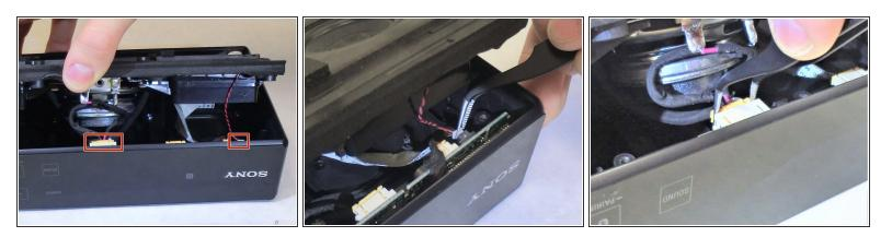
Locate the two wire connections as shown underneath of the speaker assembly and unplug them using a pair of tweezers.
