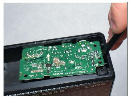
• Use a plastic spudger to remove the I/O board from the speaker body.
