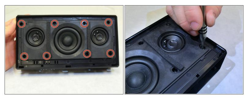
Locate the eight 8.9 mm screws on the face of the speaker assembly and remove them using a Phillips head #2 screwdriver.
