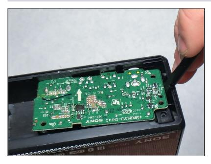
• Use a plastic spudger to remove the I/O board from the speaker body.
