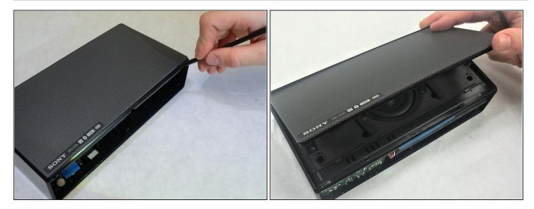
• Insert a plastic spudger into the seam of the metal speaker cover and pry it downward until it releases from the speaker body.
