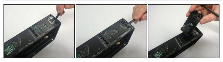
• Insert a plastic spudger underneath the edge of the input board and gently pry it away from the rest of the speaker.
