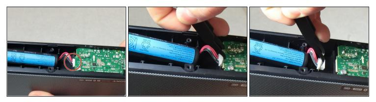
• Locate the battery plug and remove it using a pair of <u>tweezers</u>.
