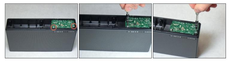
Locate the two 3.5 mm screws on the bottom of the I/O board and remove them using a Phillips head #2 screwdriver.
