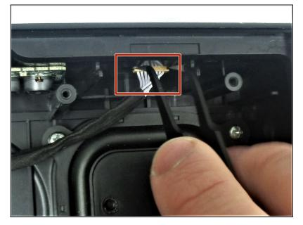
Locate the wire connecting the motherboard and the input board under the top panel of the speaker and remove it using a pair of tweezers.
