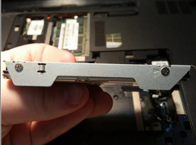
To gain access to the actual hard drive, there are two screws located on either long side of the casing that need to be undone. These screws are 3mm long and require a Phillips #1 Screwdriver to undo.
