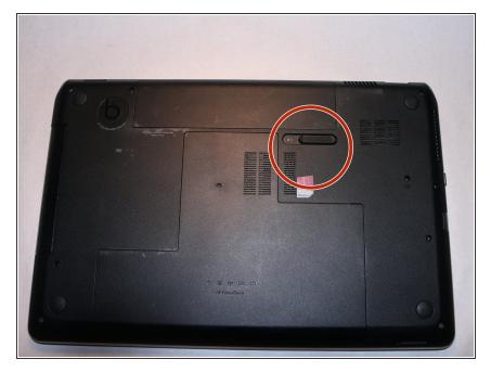
Slide the switch shown in the circle above and remove the battery from its housing. No screws are required to remove this part, and the battery should come out with little to no effort.
