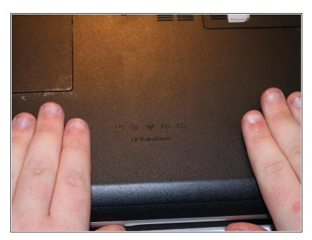
After undoing the center screw, the back cover will be able to slide off of the computer and you will have access to the inside.
