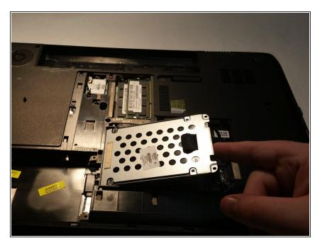
• After the screws are removed, the casing will slide to the left and then up. Make sure that the cable that connects it to the computer is as intact as possible.
