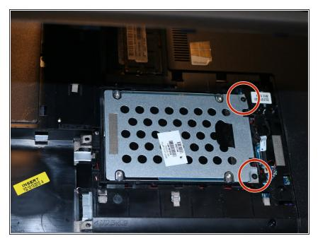
To unfasten the hard drive's casing, there are two 3mm screws that you need to undo circled above. These screws require a Phillips #1 screwdriver.
