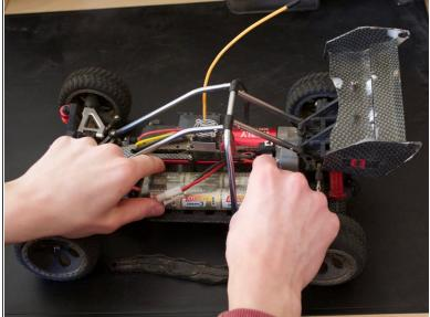
And the battery can be removed upwards
