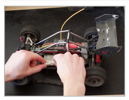
Now the battery connection is disconnected
