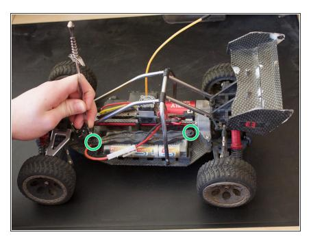
These two pins must be removed
