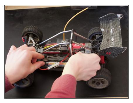
The battery holder can now be pulled off upwards
