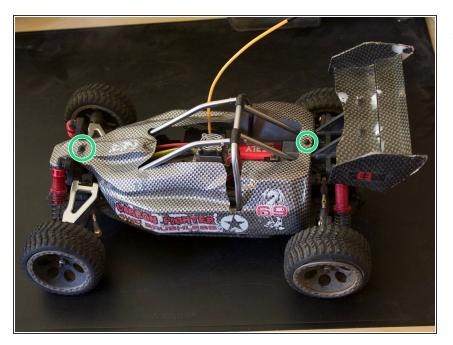
• These two pins must be removed.
