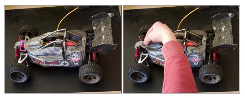
(i) TIP: if you remove the cladding more often (for example, for thorough cleaning), it may be helpful to provide the splints with some insulating tape, so the use of tools is unnecessary
