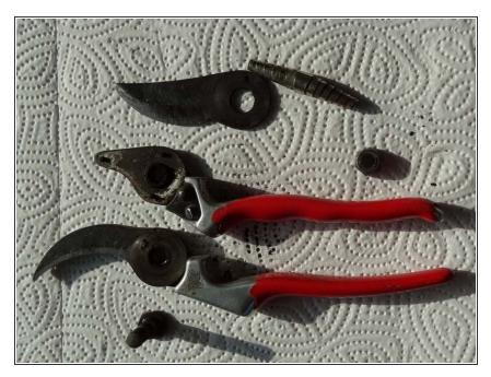
• The scissors are disassembled. We see the pivot nut, the hinge screw, the spring, the two handles and the blade.
