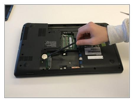
Using the plastic spudger, remove the CMOS battery, which had the letters DBV on it.
