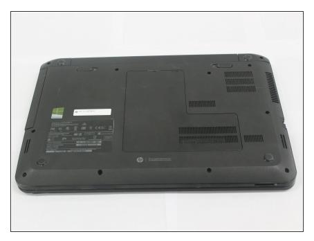
Orient the laptop upside down so that the back of the laptop, where the battery is located, faces away from you.
