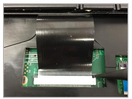
• Use your nylon spudger to release the retainer by gently lifting the retaining clips on either side.
