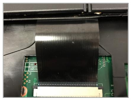
• Locate the keyboard ribbon cable, and the cable retainer keeping it attached to the motherboard.
