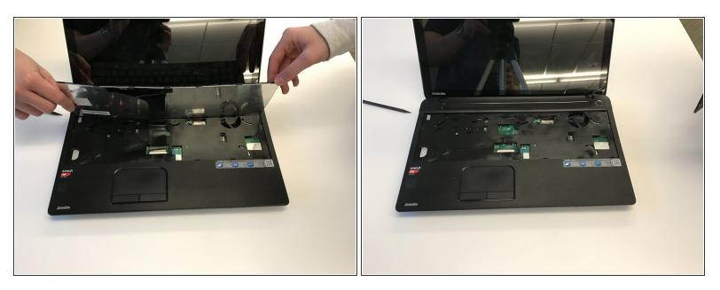
Before pulling out the keyboard, notice that it is connected to the motherboard via a ribbon cable. Gently press out the ribbon cable from its connection site and put the old keyboard aside.
