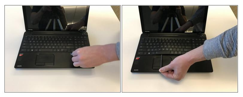
Using the spudger, go around the periphery of the keyboard while gently lifting out the keyboard little by little.
