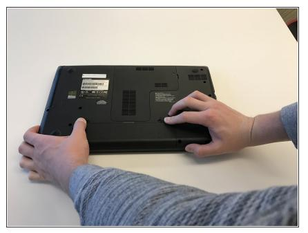
• Place fingers on the latches and slide outwards to unlock.
