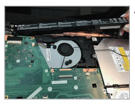
• Set the keyboard plate aside. Gently lift up battery to remove it.
