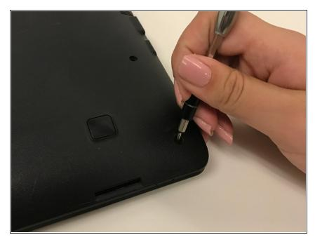
Remove all 4 mm screws using a #00 Philip's screwdriver.
