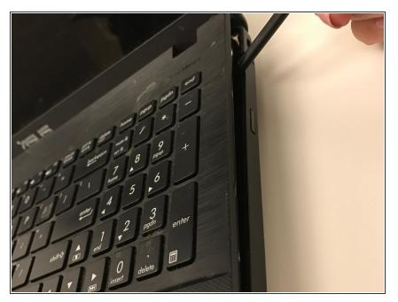
• Carefully pry up the keyboard cover with your fingers or with a plastic spudger.
