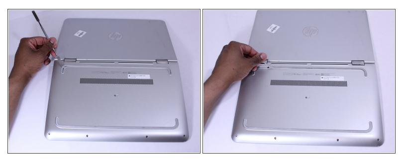
• Use a Metal Spudger and remove the rubber foot closet from the bottom of the laptop.
