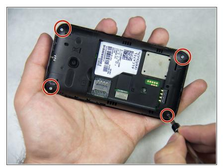
Unscrew the four 4mm JIS screws in each corner using the J000 screwdriver head. Turn the screws counter-clockwise to loosen.
