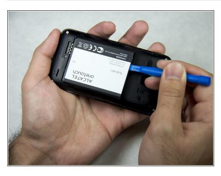
Remove the battery using one of the plastic opening tools and the domeshaped indent next to the battery face.
