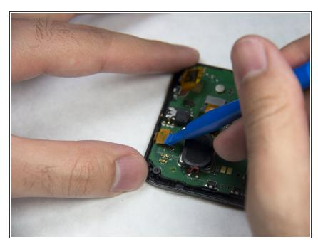
Use a plastic opening tool to lift the front camera press-fit connector free.
