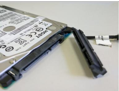
If you wish to connect the Hard Drive to an external Caddy or install it in a new machine simply remove the SATA Adapter by pulling it away from the Hard Drive
