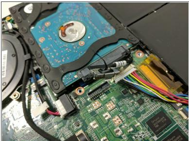
You now have access to the RAM, Hard Drive, Batteries etc. from removing this cover to remove the hard drive simply lift UP the cable that connects to the Motherboard as shown and LIFT the Hard Drive right out
