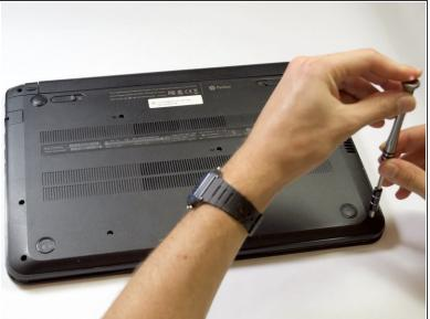
Remove the eight 7mm screws with a Philips Head #1 screwdriver.
