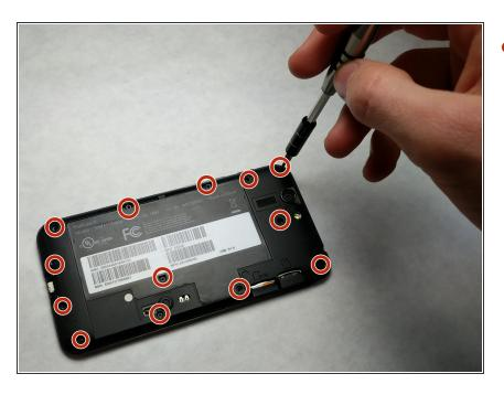
Remove thirteen 3.6mm screws using the T5 Torx Screwdriver.
