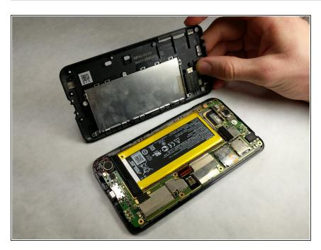
Once the screws are removed, the mid-frame can be lifted off of the phone.
