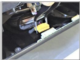
Use the tweezers to disconnect the two cables from the input board and motherboard and finish lifting the speaker assembly from the speaker body.
