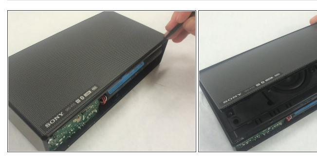
Insert the plastic sudger into the seam where the metal speaker cover meets the speaker body.
