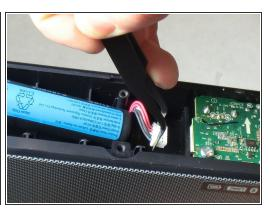
Unplug the wiring connecting the battery to the IO board using the tweezers, then remove the battery.
