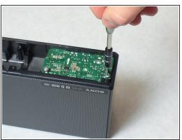
• Remove the 3.5 mm silver screws on top of the I/O board using Phillips head #2 screw driver.
