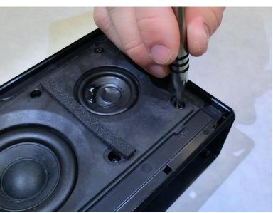
Remove the 8.9 mm screws holding the speaker assembly to the speaker body using Phillips head
