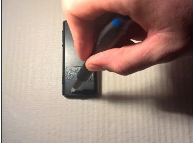
Unscrew the two Phillips screws on the back of the drive.
