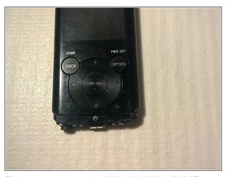
Remove the single Phillips screw that holds the front panel and the interior components of the drive.
