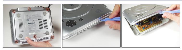
Remove the six 1cm screws on the bottom of the device with the Phillips #1 screwdriver.
