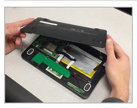
Remove the cover off the back of the device.
