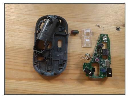
• The PCB is only held by a few clips and can be easily removed.
