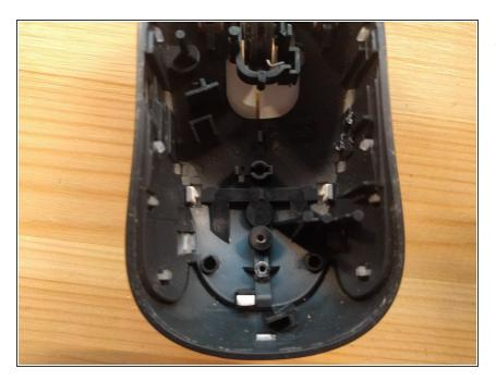
The top mouse cover can be removed by undoing three white clips holding it on the grey plastic part.
