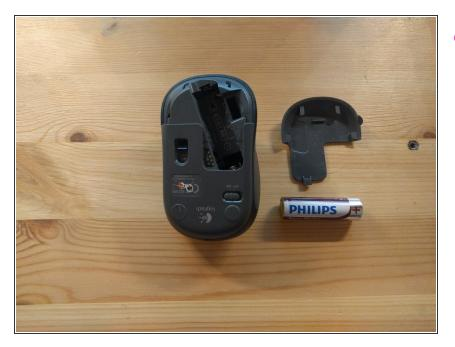
Remove the battery and battery cover
