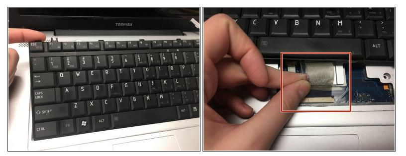
Remove the keyboard slowly. It will be attached to the laptop by a plastic connector, which can be disconnected from the laptop by pulling gently.
