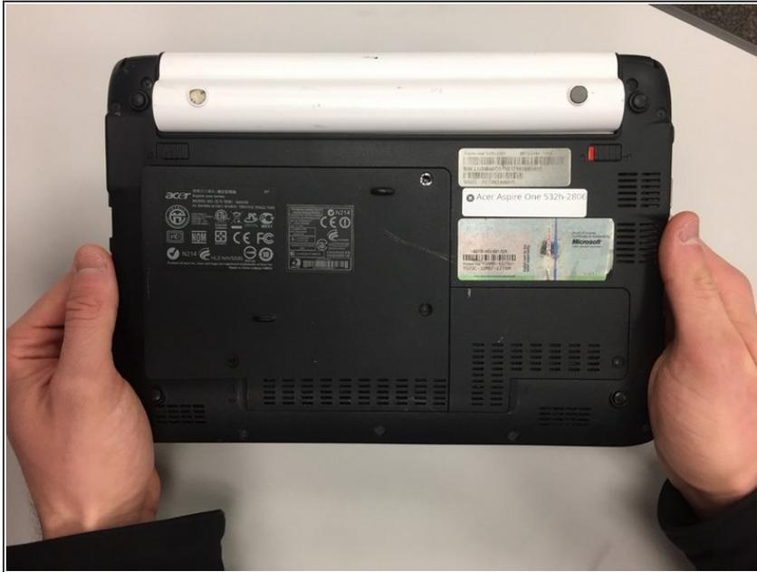
**⚠** Make sure the Acer Aspire One 532h-2806 is powered off and disconnected from any power outlets.
