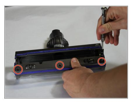
Unscrew the three front 1.4 cm torx screws using the T8 Torx screwdriver.
