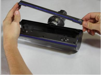
Remove the upper plate once the padlock is unlocked.
