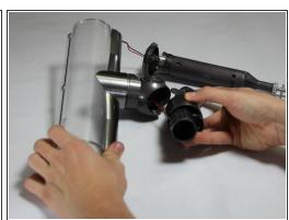
Pop off the circular plating to remove the housing from the connection piece.
