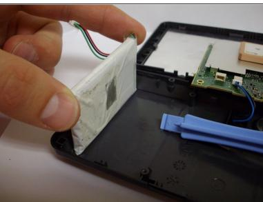
Using the plastic opening tool as a wedge, pry the battery from the case. This can be fairly tough
