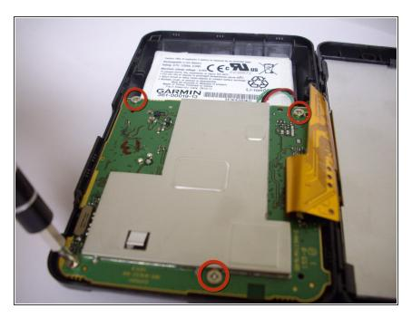
Unscrew the four 6.70 mm screws holding the motherboard in place using a philips #0 screw driver.
