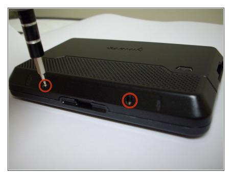
Remove two 8.4 mm T5 screws from the bottom of the device.
