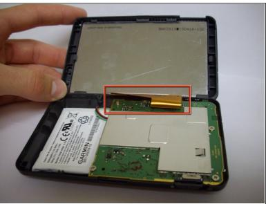
Using a plastic opening tool, carefully pry open the device.
