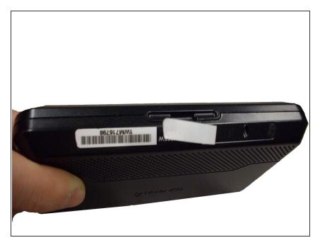
Remove the barcode sticker at the bottom of the device.
