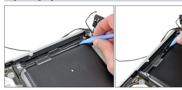
• Use a plastic opening tool or another thin prying object to carefully pry the right speaker up from the adhesive securing it to the upper case.
