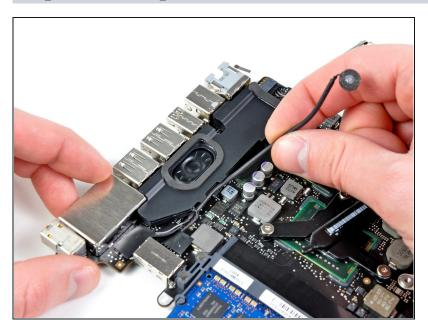
De-route the microphone cable from the channel molded into the left speaker housing.
