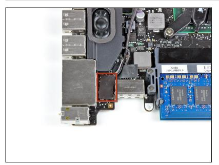
Remove the small piece of black tape covering the microphone connector.
