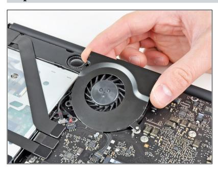
Lift the fan out of its recess in the logic board, minding its cable that may get caught.
