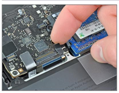
If present, remove the small strip of black tape covering the keyboard backlight cable socket.
