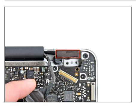
Remove the piece of foam tape covering the display screws near the MagSafe DC-In board.
