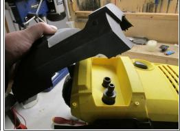
Remove the four marked Torx TX16 screws, then remove the screws from the small side cover.
