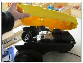
To disassemble the yellow front hood 6 cross head screws must be removed on the back. Also at the bottom, in the middle and on top. To reach the middle screws a 110 mm long screwdriver is necessarry. Turn the device and the yellow lid can be removed.
