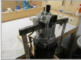
This step is important because, if the top metal bracket is removed without backup, the whole pressure springs of the thrust management come out and it will be very difficult to get them back together. I've taken long two screw clamps holding together the lower straight thrust Guide
