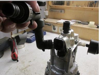
Remove the securing clips to remove the suction connection and the connection of the pressure side, then the ports can be situated. The inlet side goes out somewhat hard, there must be a little.
