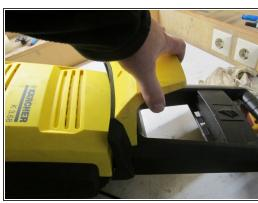
First, the detergent dispenser must be removed, to the hose at the marked position must be removed, turn the container by slightly be removed. Remove the handle Assembly to the markedcross-head screws must be unscrewed, then the handle element can be pulled off to the front.
