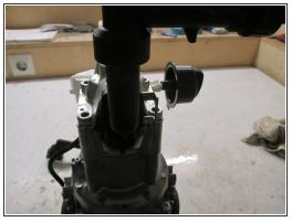
Unsrew the Screws of the motor holder flange and remove the flange, then the strain relief of the cable from the mounting brackets side out, so that the engine is now freely be removed
