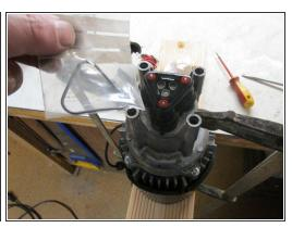
Loos the four 6 mm Allen bolts and remove the metal lid, then the head carefully remove because among them are also feathers. If necessary also the seal (90814220) can be changed in this context
