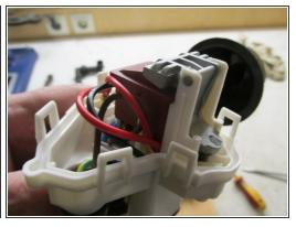
The E-box can now be pulled off upwards. The protective earth conductor must be unscrewed from the housing. You can disassemble the E box also by pushing on the clip mounts and the hood then away, how to get on the inside. The E-box comes just completely, so that it can then be replaced In order to turn the screws of the hood to sitting very deep, again, it is advisable to magnetize the screwdriver.
