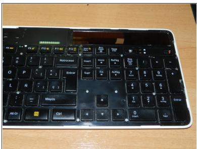
After removing the cover, the screws are visible
