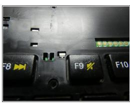
Carefully pry up the tabs around the keyboard body. Between the F8 and F9 keys there is another tab. To open it, raise it a little from below and lever it with the screwdriver, as if we were going to screw.
