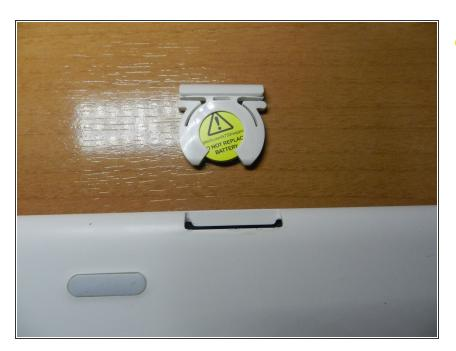
Carefully remove the battery by levering it with a flat screwdriver
