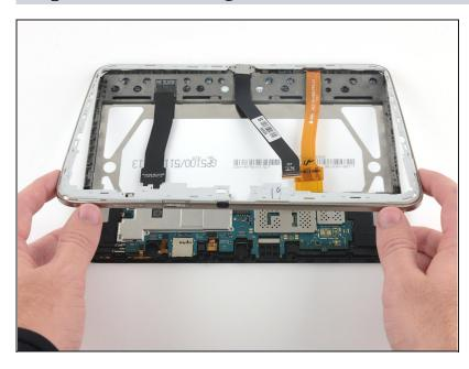
• Lift the plastic frame to remove.
