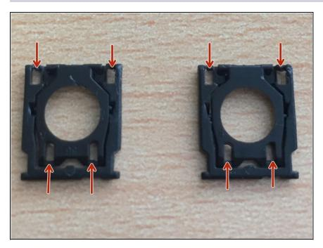
Check the plastic brackets for damage in these areas.
