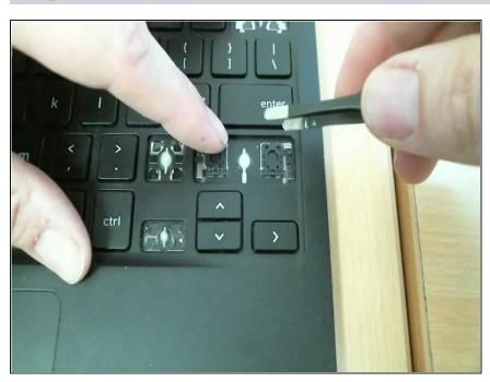
With tweezers, carefully start picking near the four corners where the 4 metal clips are securing the plastic bracket. Remember these special keys have 2 plastic brackets to remove.
