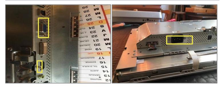
Remove the screws from the power socket of the HDMI, VGA and DVI ports if there are any.
