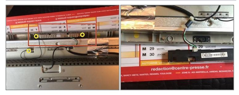
• Disconnect the various connectors, take the small Phillips screwdriver, remove the webcam and disconnect it.
