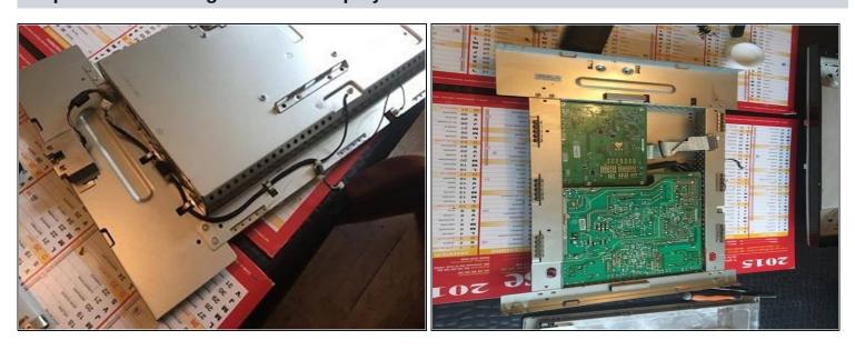
Once the tablecloth is disconnected, you can remove the metal cover from the screen. Well done the hardest part is done...
