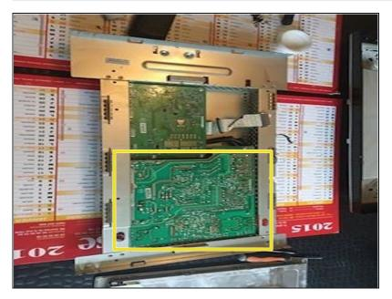
You can now remove the screws from the other electronic board (power board)
