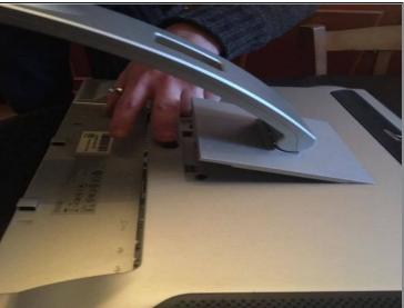
• The front panel is now completely unclipped, put the screen (screen side) against the table, being careful not to re-clip the front panel, then remove the support/stand from the screen.
