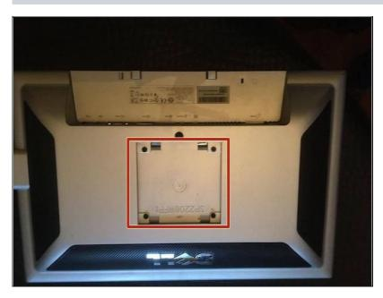
Under the fixing of the support you discover 4 large black screws. Take your big Phillips screwdriver and unscrew them. You can now remove the back cover.
