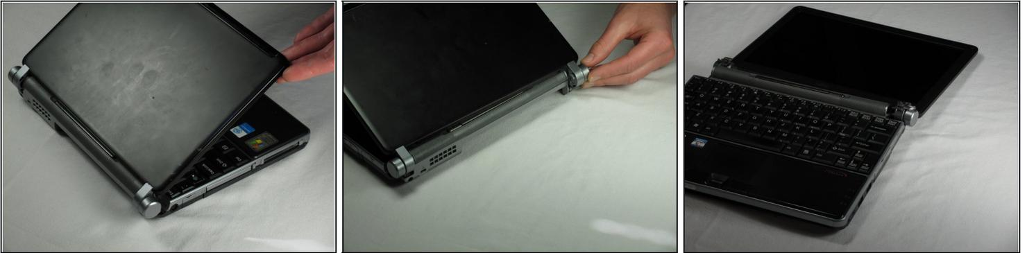
**⚠ Mind the wire connections on the bottom right side of the monitor. They are still connected between the monitor and computer.**
